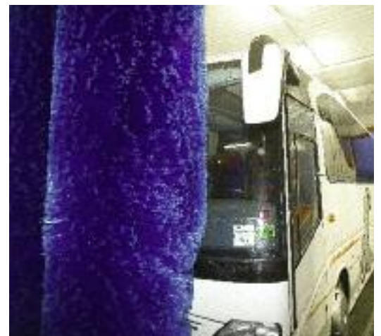
"Mirror Protection Program" (Standard on all Westmatic machines). Washes around the mirrors to prevent damage.
